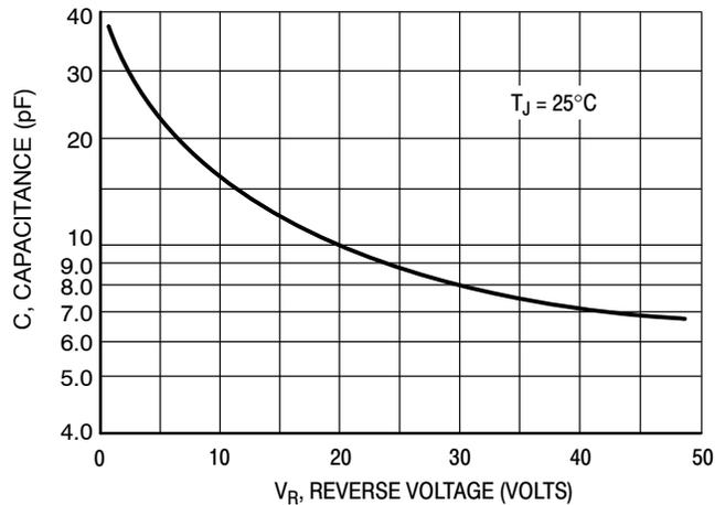
Figure 10. Typical Capacitance
