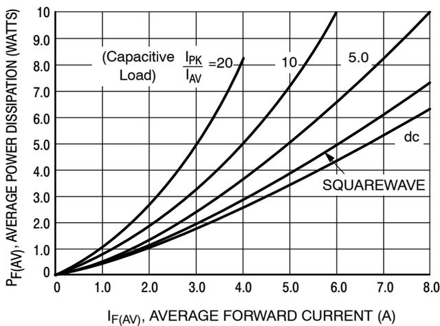
Figure 4. Power Dissipation
