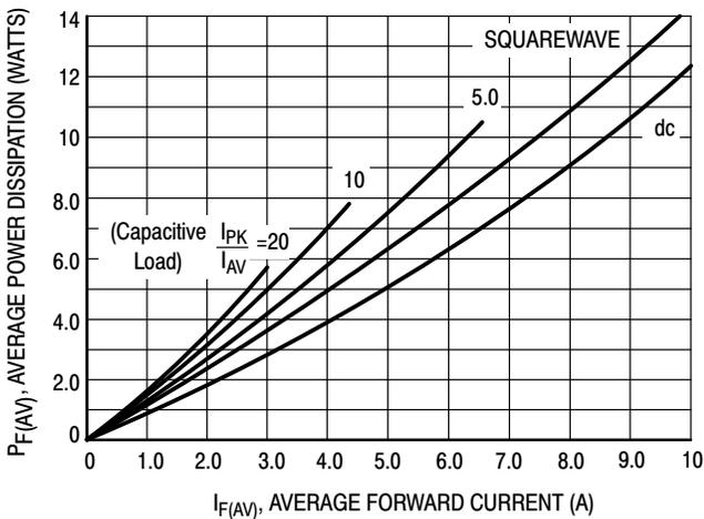
Figure 9. Power Dissipation
