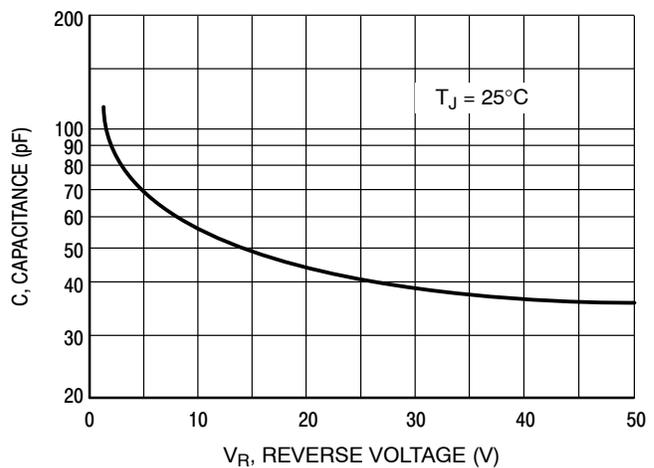
Figure 5. Typical Capacitance
